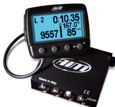
Figure 1: MyChron Light TGLog and its junction box
